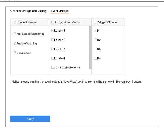
Figure 15-8 Set Trigger Cameras of POS
