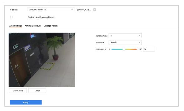
Figure 13-3 Line Crossing Detection
