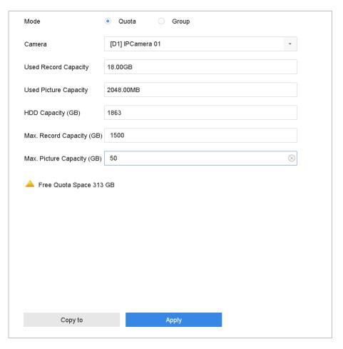
Figure 8-7 Storage Mode-HDD Quota
