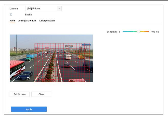
Figure 12-3 Set Motion Detection
